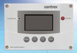
The Xantrex™ XW System Control Panel (XW SCP) features a graphical, backlit LCD display that provides system configuration and diagnostic information for devices connected to the Xanbus™-enabled network. The XW SCP gives a single point of control to setup and monitor an entire system, which may consist of multiple XW Inverter/Chargers, XW Solar Charge Controllers and other components.
